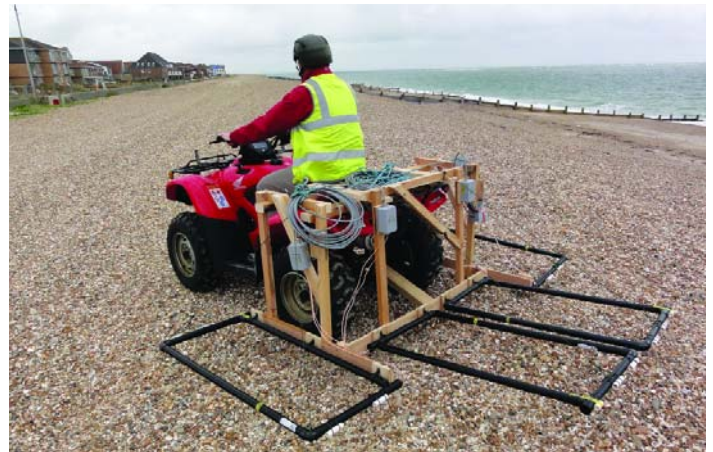
Figure 3: ATV mounted RFID antenna.
