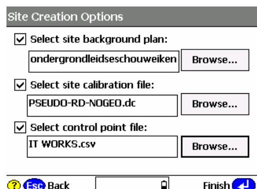
If no calibration file (DC) is at hand, it is possible to calibrate the site using the known points in the .csv file. Simply select calibrate site in the [Systems Setup](#) menu
