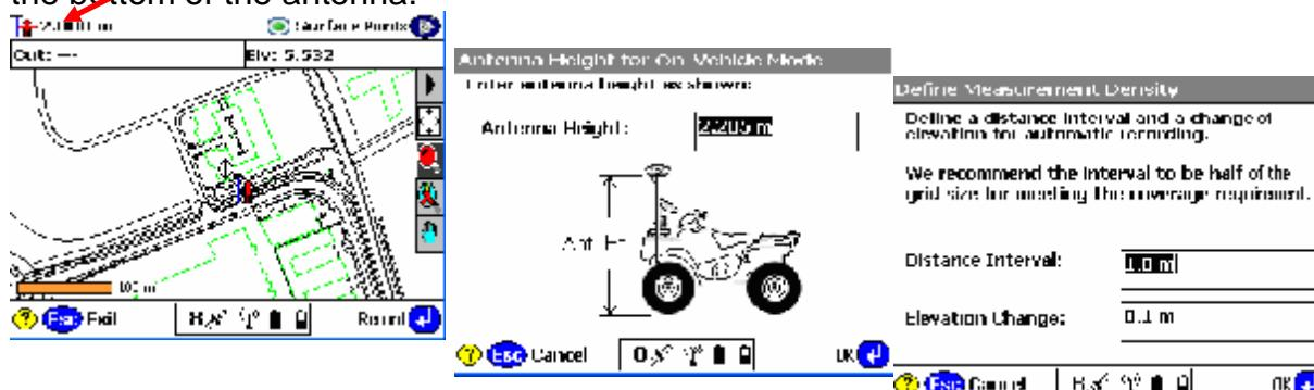
Finally select the measurement density required for the job, this will make the system log at a minimum interval or elevation change.
