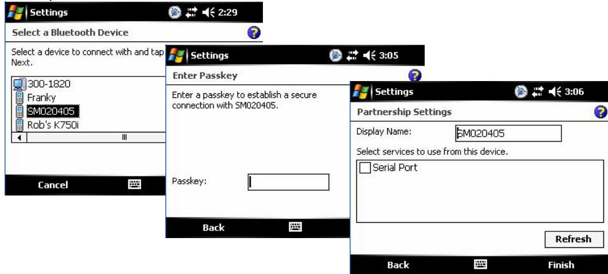
After this, the serial port has to be assigned by selecting the tab COM ports and select **New Outgoing Port**. Again select the Sonarmite and select **Next**. Now deselect (unchecked) secure connection and select **Finish**.
