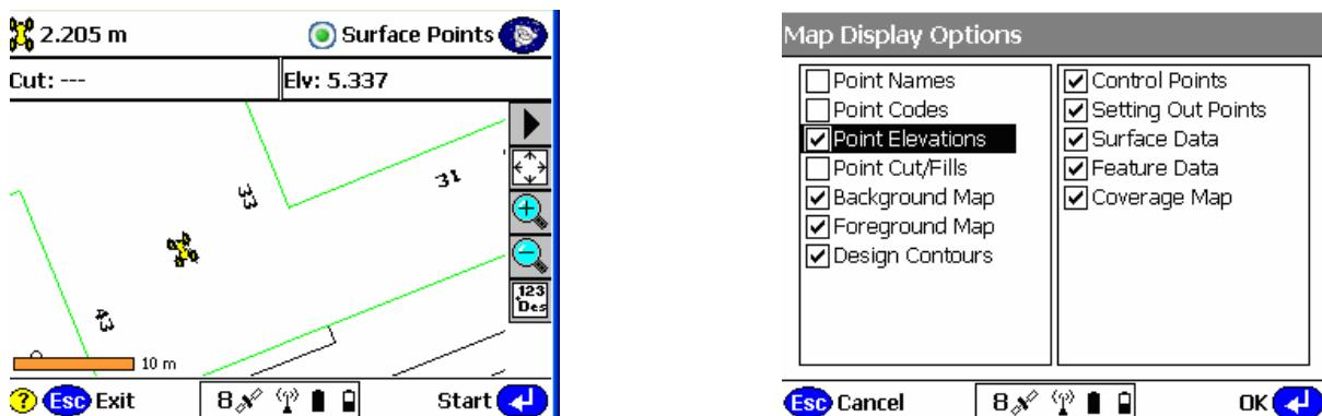
Remember that if loads of points are stored, this option can slow down the CE device and make the map hard to read, so switch off again if required.
