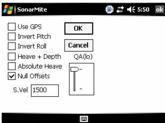
The functions that Now select **Device>SonarMite** and select the previously assigned COM port (in this case COM 8) Leave the other settings as per default (9600,8,n,1 no flow control) Select **OK** and the echo sounder should now return depths. It is possible to fine-tune the Quality threshold, it is advised to leave it low in order to pass all data. Leave the SonarMite software running and continue with the next part. If you encounter problems (unable to connect etc) reset the TSC2 (swIn this
