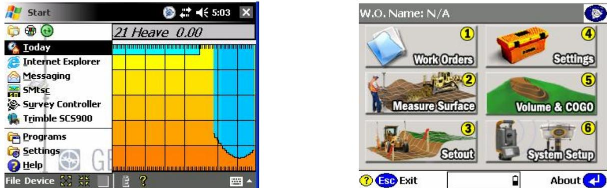
In the new site, the various files are selected, a minimum is the site calibration file (DC file) in order to get the proper coordinate system, or a csv file containing control points (Since it is recommended to check the system setup, a .csv file is important). Currently this site calibration can contain a Geoid model, but CAN NOT contain a shiftgrid!..
